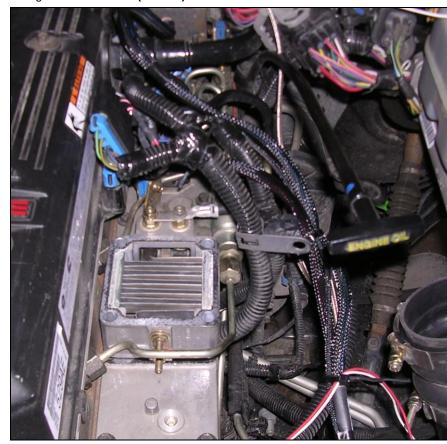
Place the new gasket (supplied) in place on top of the intake heater.
